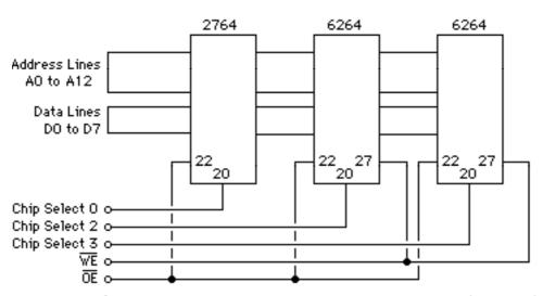
Pins 26 & 28 Connected to +Vcc. Pin 14 Connected to Ground (All chips)
